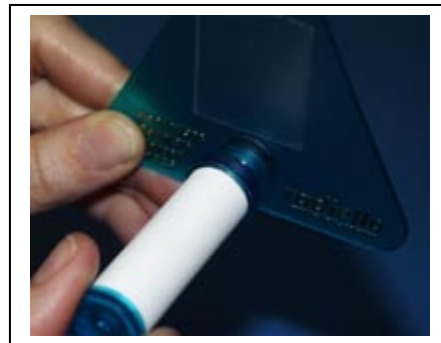
Installation of sampler onto support plate
